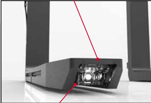
High quality camera with LED lights completely integrated in the fork tip
