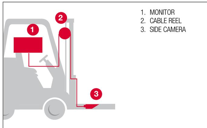
The Easy-Fork Vision Systems range includes the Side fork camera, the Tip fork camera, and a modular solution to be installed on the fork carriage including Front camera and laser.
