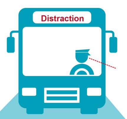
When the driver's line of sight deviates from the driving direction, the system will automatically give sound and light alarms.
